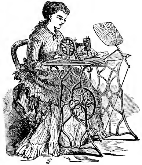
Figure 65.—THIS FANNING ATTACHMENT was commercially available from James Morrison & Co. in the early 1870s; it sold for one dollar as stated in the advertising brochure from which this engraving was copied. Other inventors also patented similar implements. (Smithsonian photo 45513.)
